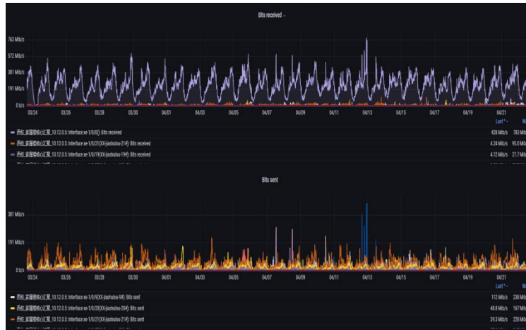
Fig. 9: Network device port traffic monitoring based on SNMP
